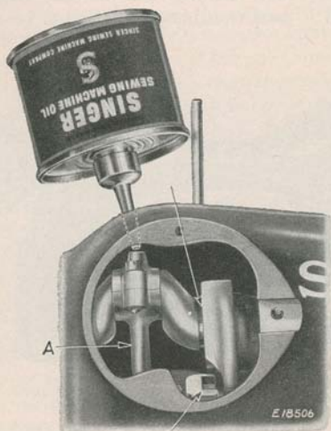
FIG. 24. OILING POINTS AT THE BACK OF THE MACHINE
