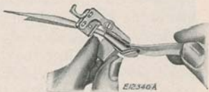
FIG. 43. INSERT FOLDED BINDING IN OUTSIDE SLOT
