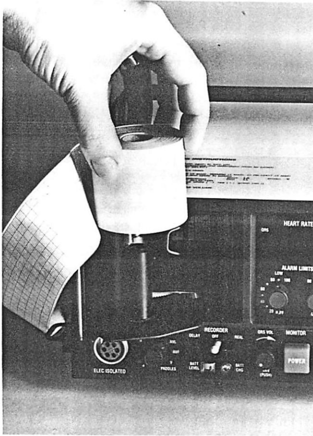
Figure 2-5 Recorder Paper Replacement
