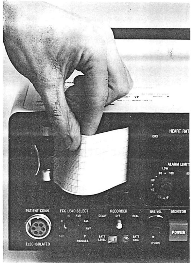
Figure 2-5 Recorder Paper Replacement
