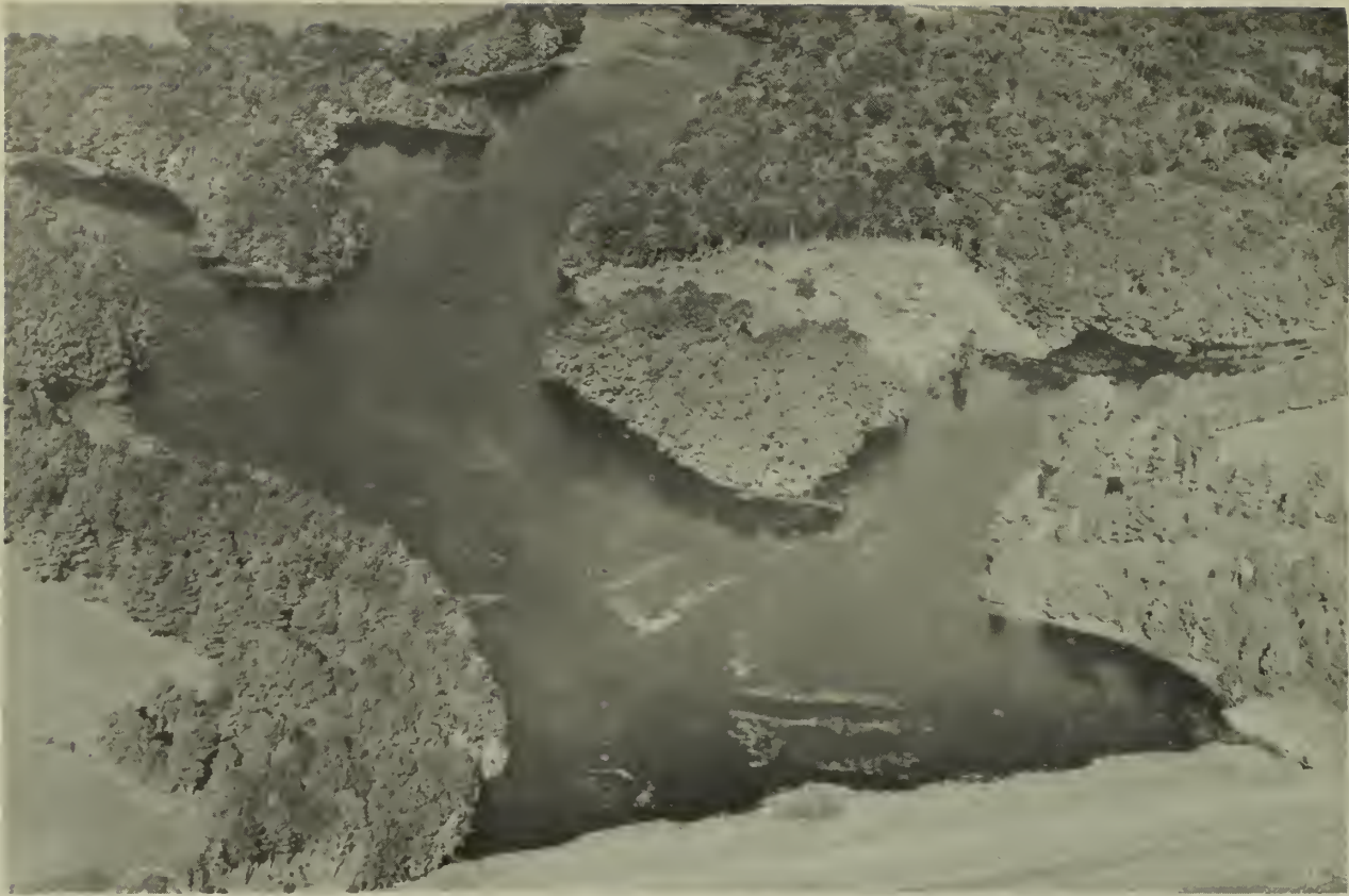
Figure 7. —Highway pond above Portsmouth, N. H., where new turnpike was used as a dam to impound a former salt marsh. Outlet structure, which includes a fishway, is shown at extreme lower right. The development resulted in substantial benefits to fish and wildlife.
